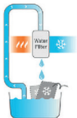
Traditional evaporative air cooler
